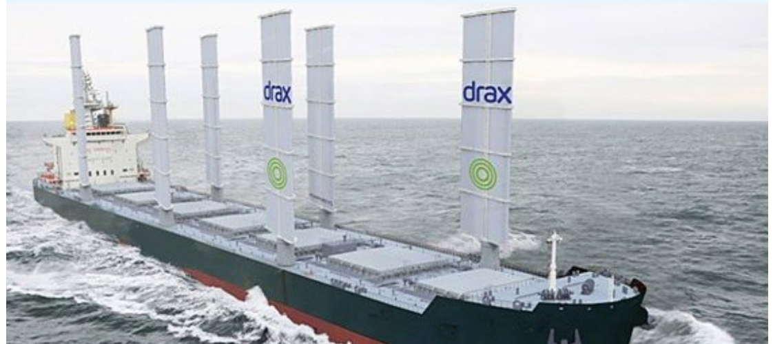
Visualisation of FastRigs installed on a dry bulk ship© Smart Green Shipping
