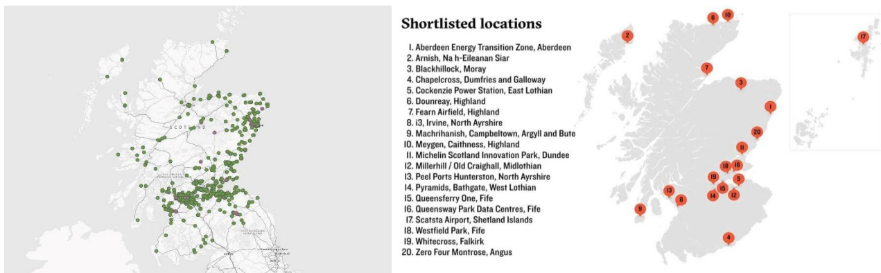
Figure 2. Existing District and Communal Heat networks 8 (green, left) vs Shortlisted major planned Data Centre locations 9 (orange, right) in Scotland
