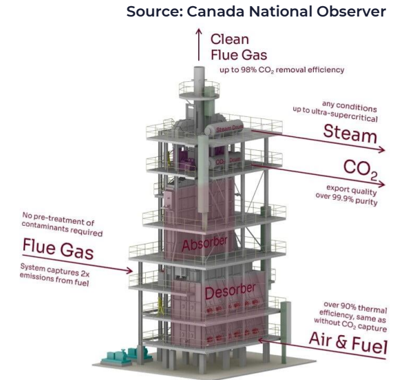
Fig 4.5-2, Photo of the Kruger pulp and paper plant with demonstration carbon capture project, alongside a Mantel Capture system
