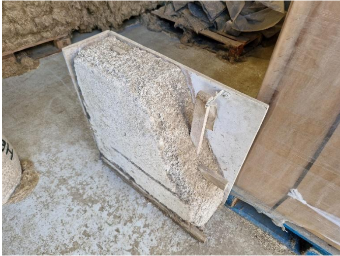
Fig 31 Demonstration of shiv used for shuttered hempcrete walling at Harrison Spinks
