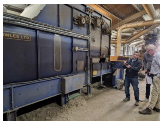
Fig 26 Decortication equipment at East Yorkshire Hemp
