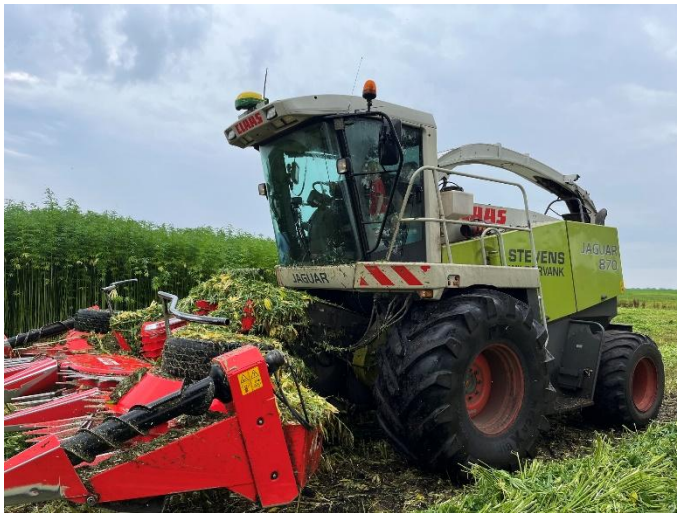
Fig 21 Claas forage harvester with Kemper header for cutting hemp crop
