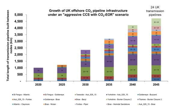
Figure 34: Growth in  $CO_2$  pipeline infrastructure for the Aggressive CCS with  $CO_2$ -EOR scenario. Each colour reflects different network nodes. Figures inside the bars reflect the diameter of pipelines (in inches).
