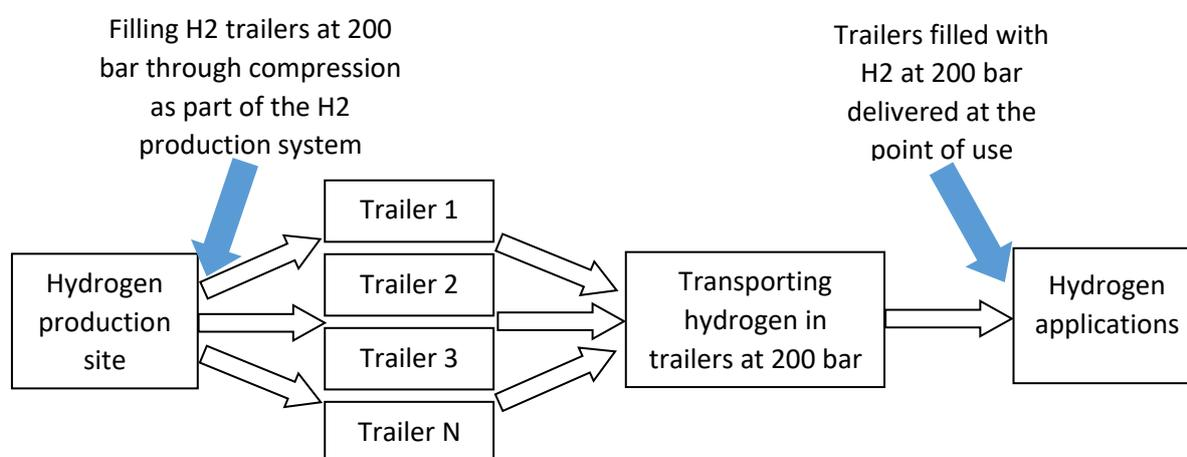
The aim of this scenario is to identify the cost for transporting hydrogen from the point of production to the point of use.
