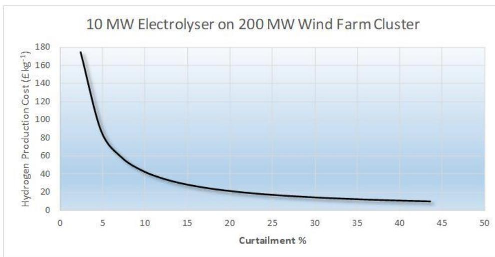
The cost of electrolysis is extremely high for low curtailment. For example, a 10 MW electrolyser operating at full power for 1.5% of the time uses 1300 MWh of electrical energy a year. This is enough to make 20,000 kg of pressurised hydrogen (assuming 65% electrolyser efficiency and 60% for the overall hydrogen system) a year.
