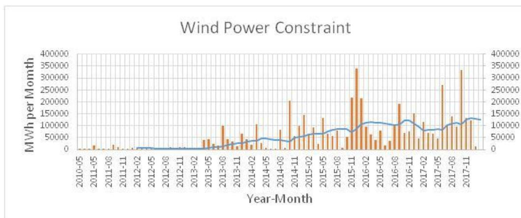
Note that the amount of electricity generated from wind turbines is increasing each year. As such the above graph shows that the fraction that is constrained is actually decreasing in comparison to the overall increase in wind generation capacity.
