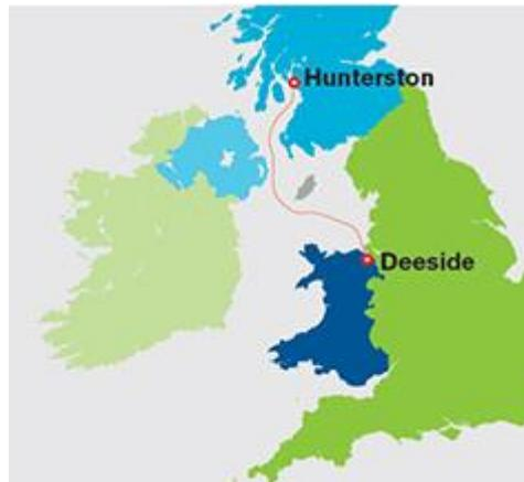
The 2200 MW link will provide several benefits including strengthening the transmission network. Most relevant to this study is its expected effect in alleviating constraints on the Scottish network by transporting large amounts of energy from the Central Belt down to demand centres in England & Wales.
