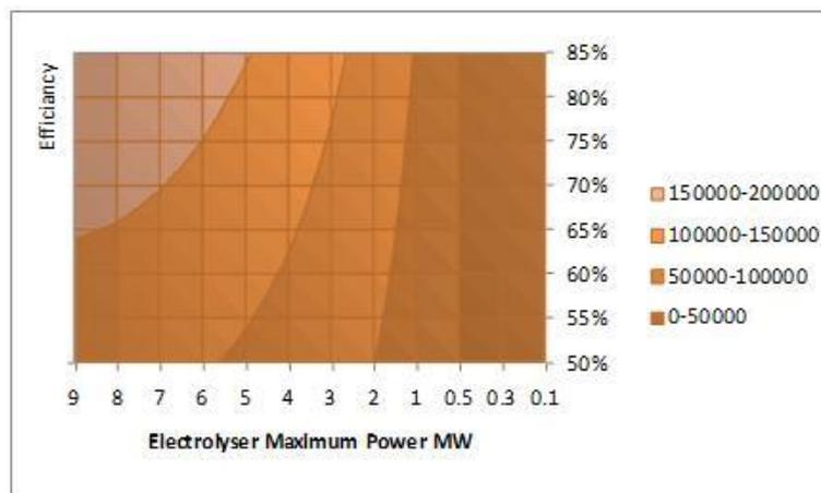
From Figure B.3, it is possible to identify the region where the electrolyser versus income is optimised. In this particular case, a reasonable configuration to take forward into a cost analysis is a 3 MW electrolysis capacity with an efficiency of 75%.
