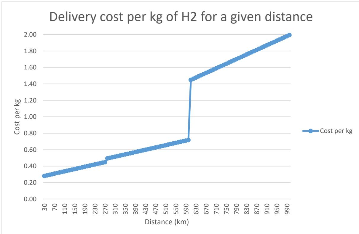
**Table 6.6 - Cost per km and cost of delivery per kg of H2 for different distances**
