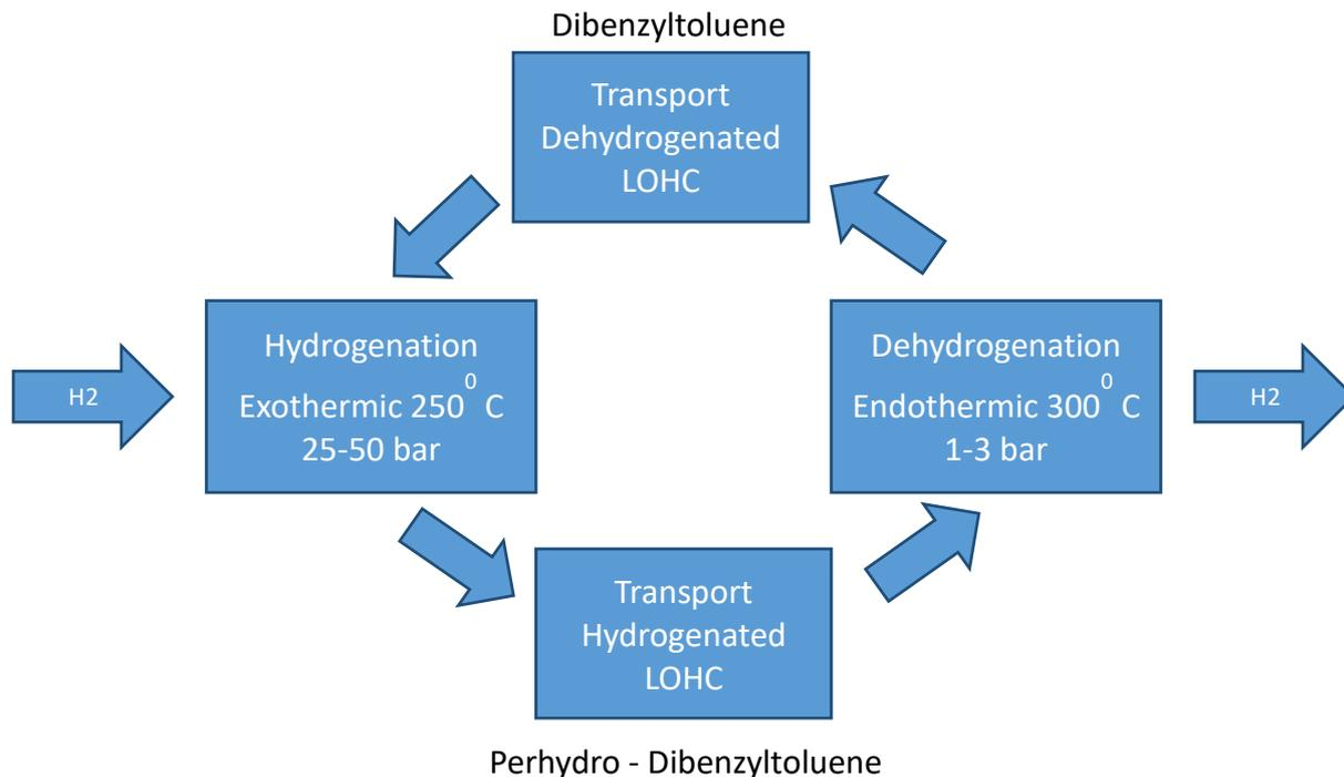
Only a few steps are required to store and release hydrogen using the LOHC technologies. First, when hydrogen is produced, it needs to be pressurised up to 50 bar (lower pressures are also possible depending on the technology being used).
