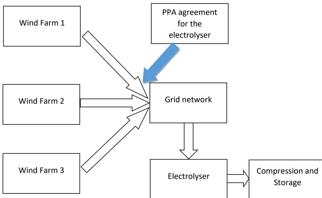
The aim of this scenario is to investigate the possibility of purchasing electricity in order to run the electrolyser for most of the time during the year. The scenario must not be confused with Scenario 3 where the selected electrolyser was scaled to match the size of a single wind farm.
