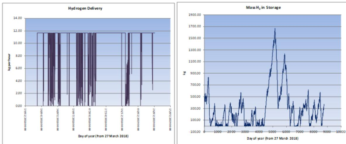
Figure 5.23 shows that there is a shortage of hydrogen in the summer. It also shows that the tank has storage capacity not used over a long period of time during the year. The graph on the left illustrates the quantity of hydrogen that is delivered to the end user and that without large scale hydrogen storage; the ability to meet the end demand is compromised.
