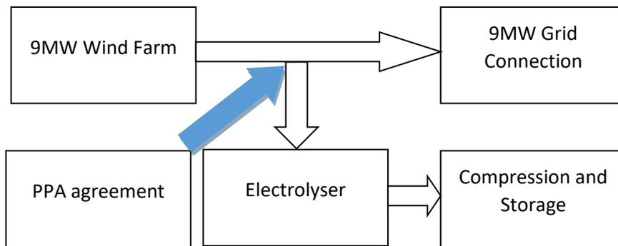
The aim of this scenario is to investigate if the purchase of electricity from a 9 MW wind farm with moderate constraint at their existing PPA price of £33 MWh<sup>-1</sup> is financially viable for a hydrogen system.
