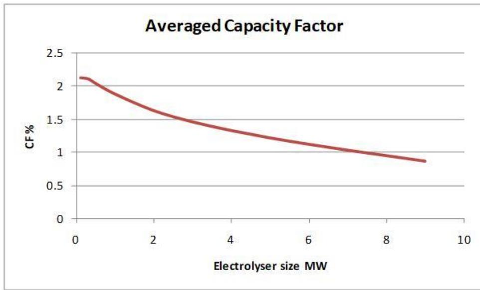
As Figure B.2 shows, the electrolyser capacity factor for this wind farm is very low. Using the previously stated assumptions (£5 per kg of hydrogen, £1 per kg of oxygen, £20 per MWh of heat) it is possible to calculate the annual income. This is shown in Figure B.3.
