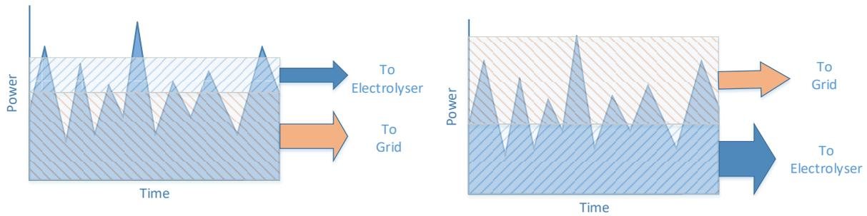
On the left of figure 5.9, the electrolyser only takes the curtailed and highly variable power. On the right, the electrolyser has a priority despatch contract, meaning it takes the cleanest and most available power off the wind farm.
