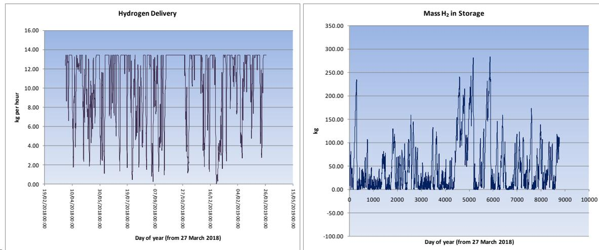
In this case, there are several periods when there is insufficient hydrogen (see Figure 5.24- right).
