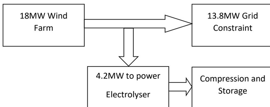
The impact of paying for the electricity on economic viability is investigated. A 4.2 MW electrolyser capacity is considered to be installed on site and is evaluated using the data from a typical year (2014).
