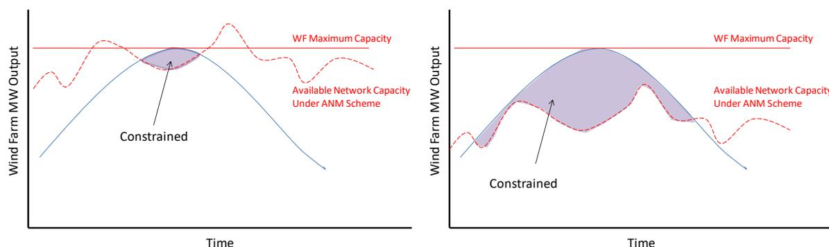
The priority stack of an ANM scheme would also play a role in determining levels of constraint, where in a last in first off (LIFO) stack, the generation connecting later would be more frequently constrained and so could benefit more from the hydrogen application than earlier connections.
