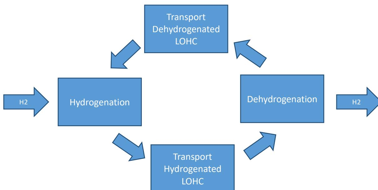
In this concept, aromatic compounds ‘absorb’ hydrogen in a catalytic hydrogenation reaction. The output compound is saturated with hydrogen and stored at ambient conditions. It is this saturated compound that is transported to the site where the hydrogen is to be used.
