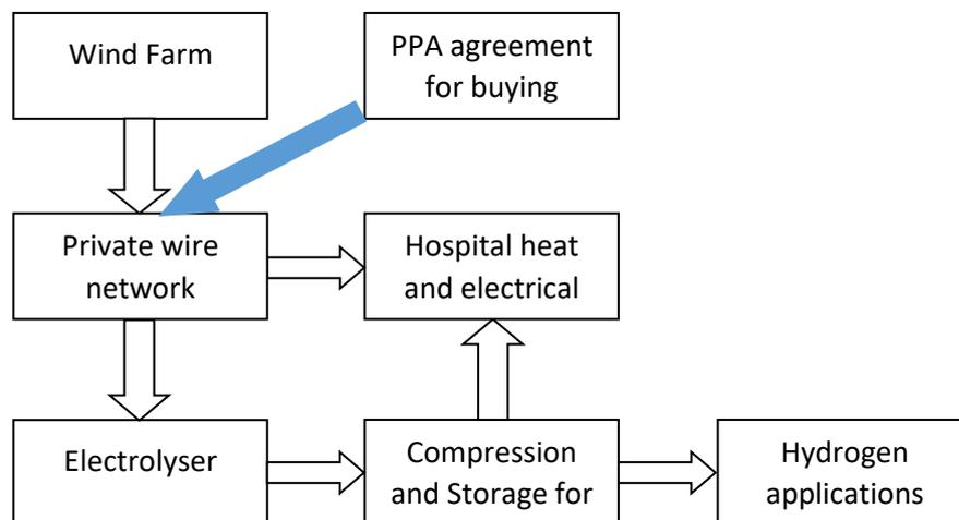
The aim of this scenario is to identify whether selling the by-products, specifically oxygen and heat, from a hydrogen facility can lead to better financial returns. The rationale behind this analysis is to investigate niche hydrogen applications (i.e. hospitals) where both oxygen and heat can be used. For those niches, it is helpful to determine how selling the by-product heat and oxygen impacts on the financial viability of a green hydrogen installation.
