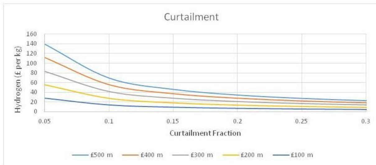
The different coloured curves illustrate the price of hydrogen per kilogram associated with a price of a given hydrogen system (including electrolyser, compressor, storage, etc.). To be more precise, for a 100MW wind farm, the cost of the hydrogen system is taken as:
