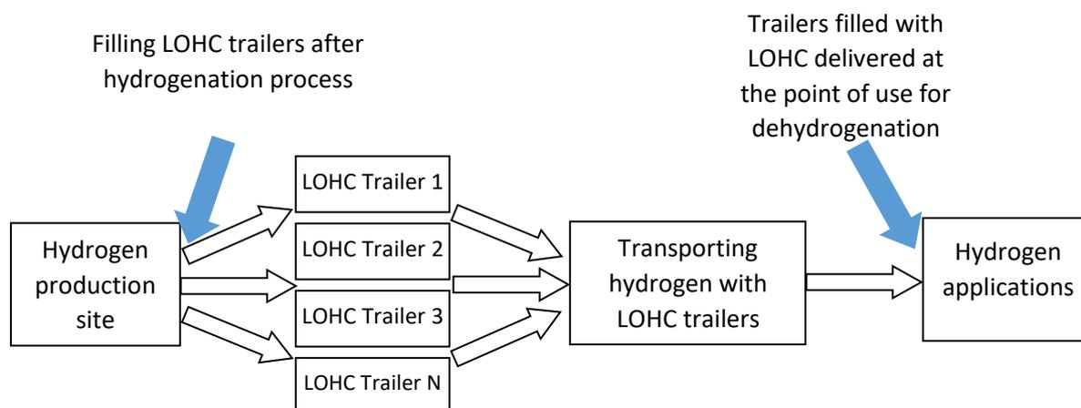
The aim of this scenario is to identify the cost for transporting hydrogen using the LOHC storage medium from the point of production to the point of use. This will be expressed in £s per km, and calculated a £s per km cost over distances of 25 km, 50 km, 100 km, and 200 km and above.
